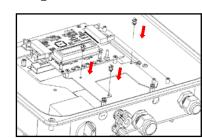
2.2.3 Plug the ComBox PCBA onto the spacer support.
