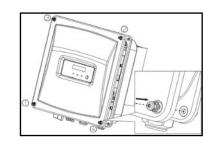
2.2.11 \*Take off the sealing cap and tighten the antenna into the WiFi connection port by hand. Make sure the antenna is securely connected.
