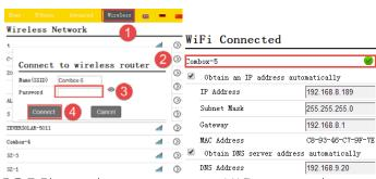
3.2.5 Please change to a secure WiFi password to ensure highest security and prevent unauthorized access, refer to manual for the process of password change (you can download the manual from Zeversolar home page <u>www.zeversolar.com</u>)
