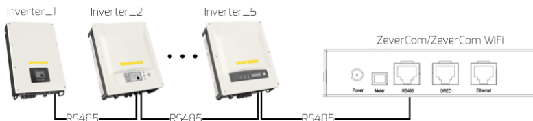
Fig. 5-2: Connection to the inverter
