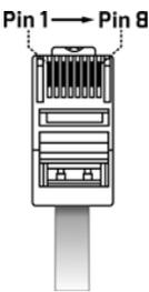
The diagram shows a top-down view of an RJ45 connector. Two dashed lines with arrows point from the labels 'Pin 1' and 'Pin 8' to the first and eighth pins of the connector, respectively.
